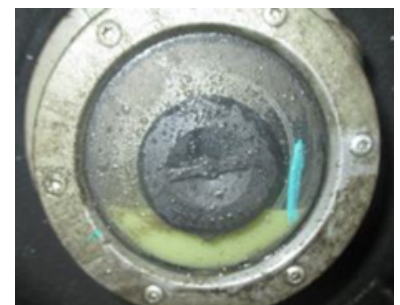
Figure 1: 50 weight synthetic oil contaminated with a small amount of water turns milky white.
