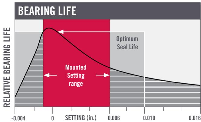
Precisely set bearing tolerances yield maximum bearing life.
