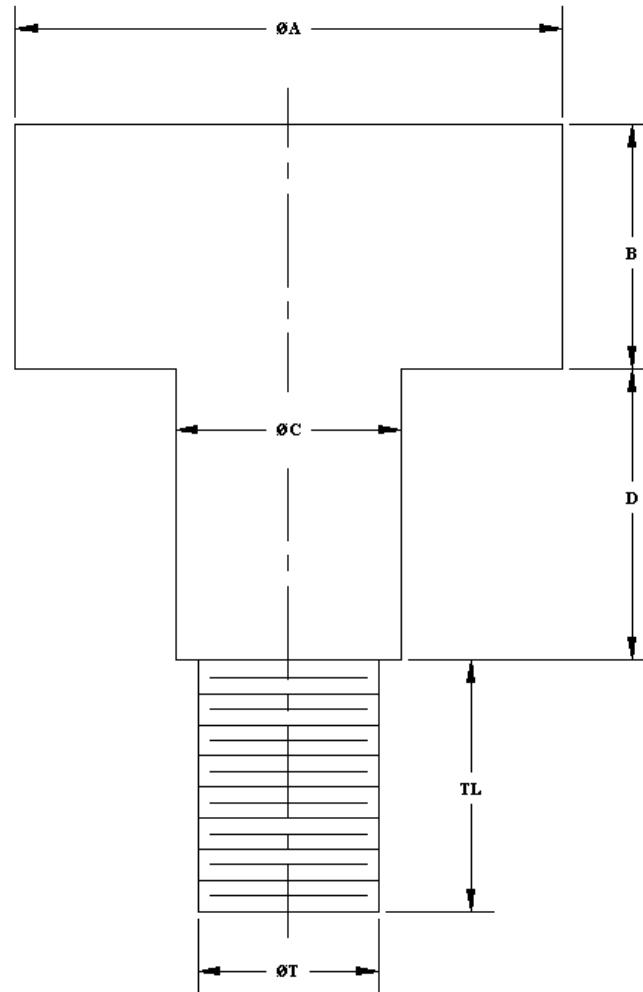
NOTE: Length of small diameter (D) to be adjusted to fit piston rod into carrier with approximately 1" of steel between large diameter ( $\text{\O}A$ ) and back of carrier.
