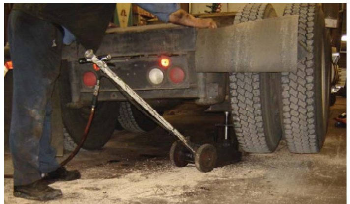
Lift axle eight inches to allow lubricant to flow into the hub on the opposite end of the axle.
