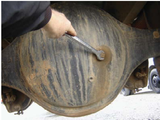
Remove plug to check lubricant level in axle reservoir.
