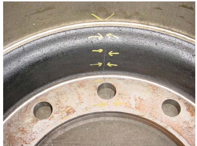
Example of drum cracking.
