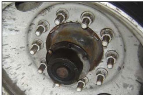
Inspecting for loose, damaged or missing fasteners and hubcaps is an important part of a driver's pre-trip routine and preventative maintenance requirements.
