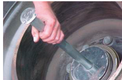
Properly seat the seal into the hub.
