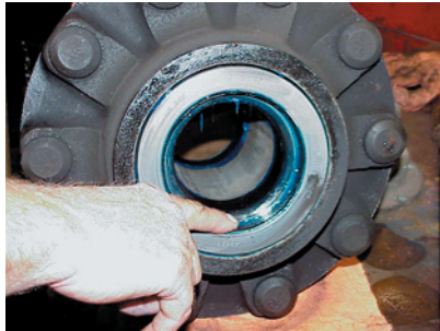
Lubricate the ID of the seal.
