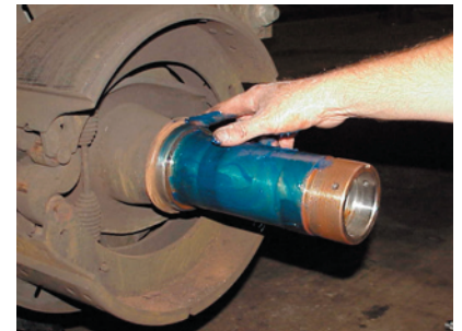
Grease the spindle prior to hub installation.
