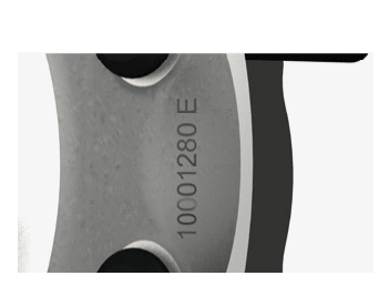
Figure 5: Casting number on the back side of the mounting flange.
