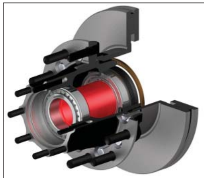
Iron PreSet Hub and U-Shaped Rotor Assembly.
