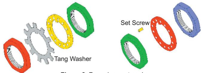
Figure 2: Four-piece nut packs.
